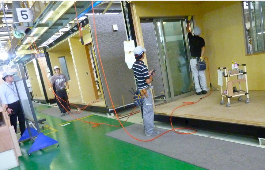
Figure 4.5 Rooms for a Toyota home built on an assembly line with the workload balanced to takt.
