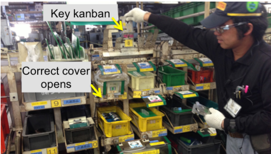
Figure 8.1 Manual key kanban opens only the cover of the correct part to pick next.
