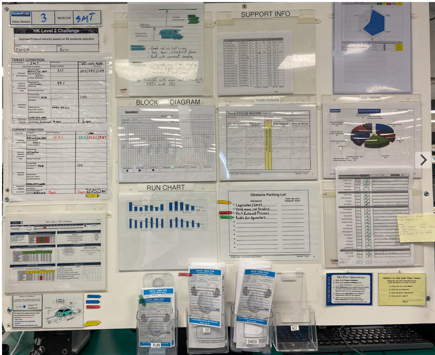
Figure 13.15 SigmaPoint Technologies L3 process level daily management board (based on Toyota Kata).
